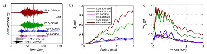
Figure 2. Input ground motions achieved on the shake table: (a) Acceleration time-histories; (b) Elastic displacement response spectra ( $\xi$ =5%); (c) Acceleration response spectra ( $\xi$ =5%).
