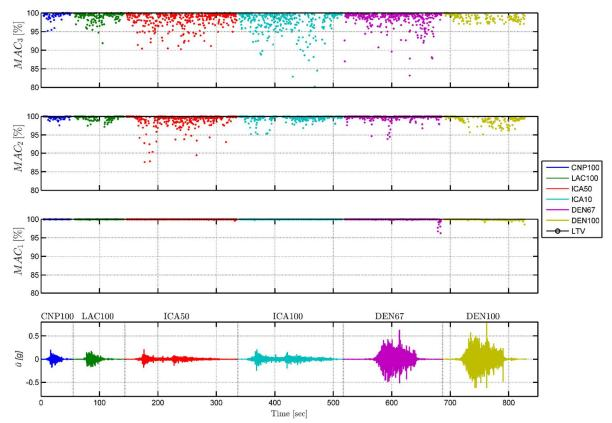
Figure 7. Temporal evolution of the MAC values corresponding to the first three longitudinal modes.
