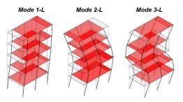
Figure 4. Identified mode shapes of the building.
