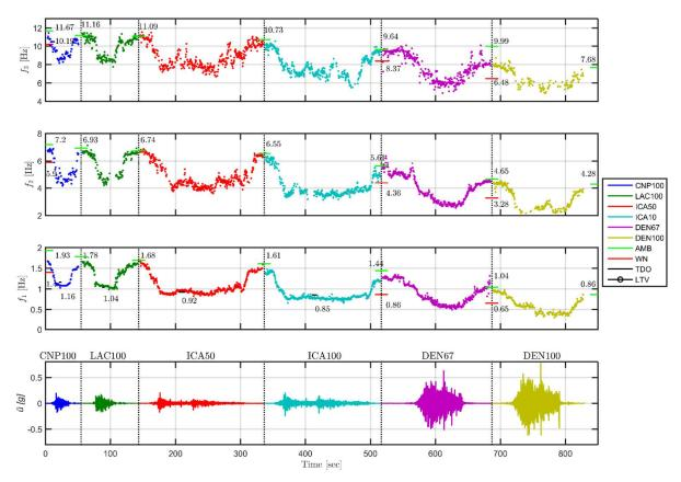
Figure 5. Temporal evolution of the natural frequencies identified for first three longitudinal modes.
